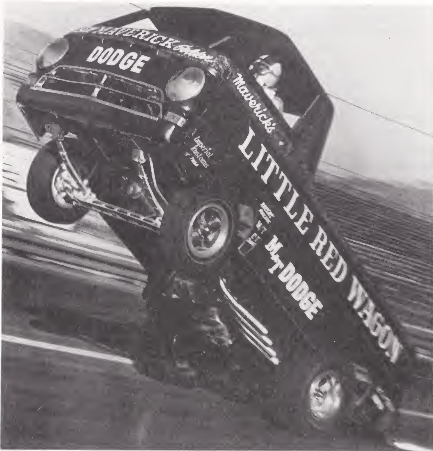
Exhibition machines like Bill Golden's "Little Red Wagon" were designed to pull the front wheels up as soon as they left the starting line and to keep them up the full quarter-mile, like this. (Courtesy Bill Golden)
