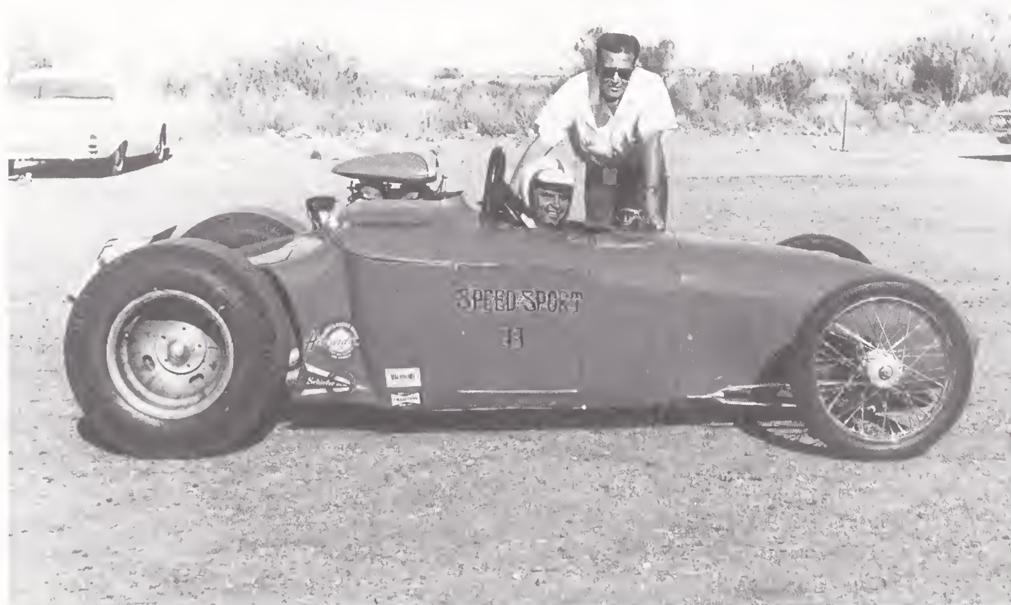
Red Greth and Lyle Fisher (in cockpit) pose with their "Speed Sport" roadster, in its second incarnation in the early 1960s. Contrasts with the Henslee machine include a narrowed rear axle, supercharger, parachute for stopping, and roll bar for insurance. (Photograph by Bill Turney)
