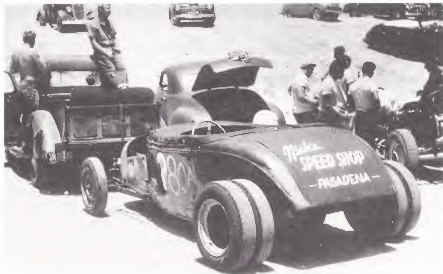
The Nicholson brothers' "?"—a coupe from which the top had been removed—is seen here in 1951 at the Paradise Mesa strip, near San Diego. The paired tires were an attempt to enhance traction. At right is the old lakes machine that became Art Chrisman's first dragster (see page 20). (Courtesy Don Montgomery)
