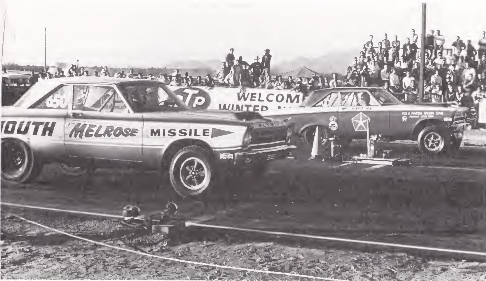
The cars are both Plymouths, but the wheelbase alterations to Ronnie Sox's (far side) are readily apparent. Sox's was one of the machines from Chrysler which gave rise to the appellation "funny car" (but compare with photo at left ten years before). (Photograph by Bill Turney)
