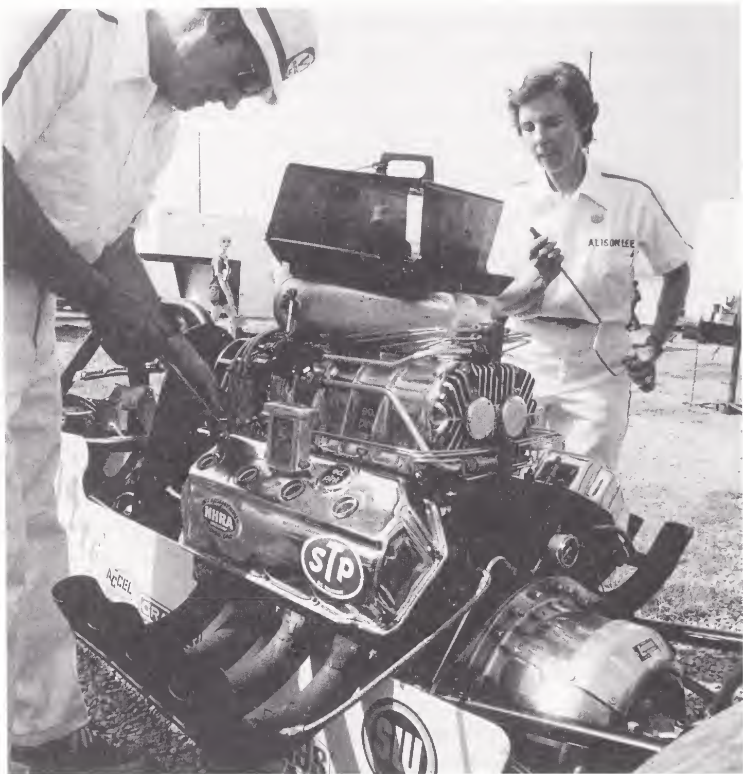
Jim and Alison Lee, husband and wife from Warrenton, Virginia, were fixtures on the top-fuel scene from the mid-1960s to the mid-1980s. Here, at the NHRA Springnationals near Columbus, Alison is checking spark plugs, while Jim removes a rocker arm cover from their Ed Pink hemi. (Author's collection)
