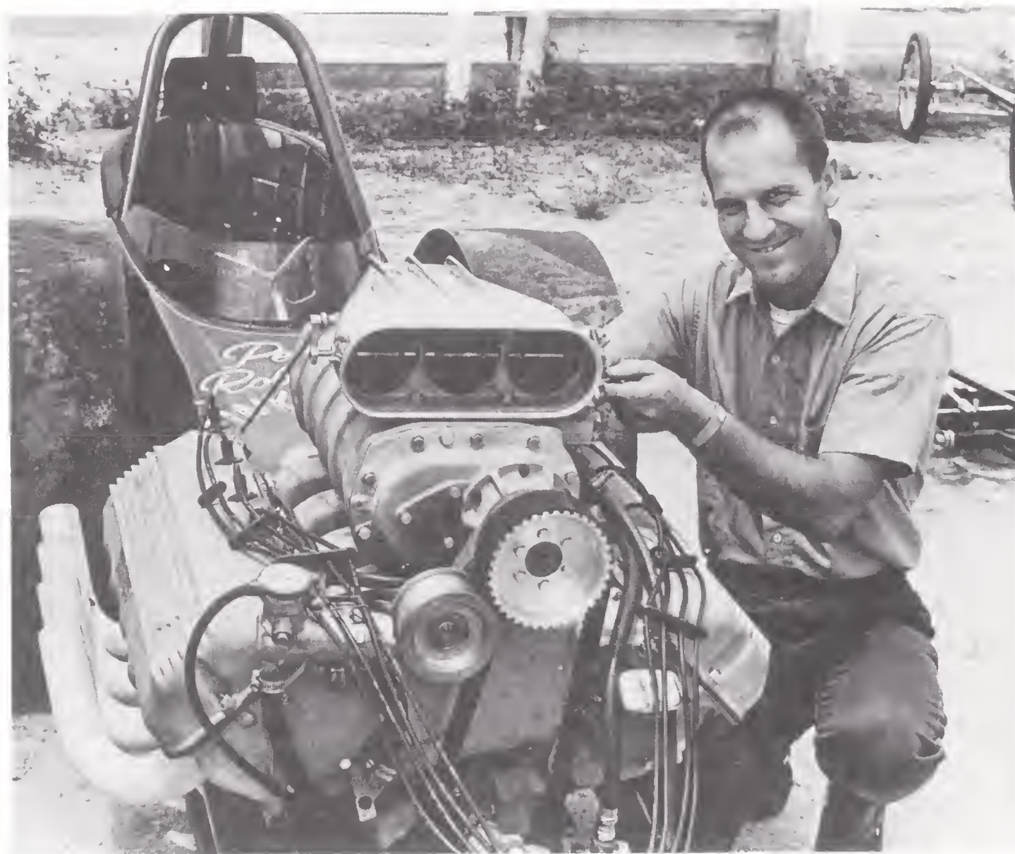
Pete Robinson pauses for a photographer as he works on his single-overhead-cam Ford engine. Robinson manufactured various components for use when these engines were converted to superchargers and nitro, including blower drives. (Author's collection)
