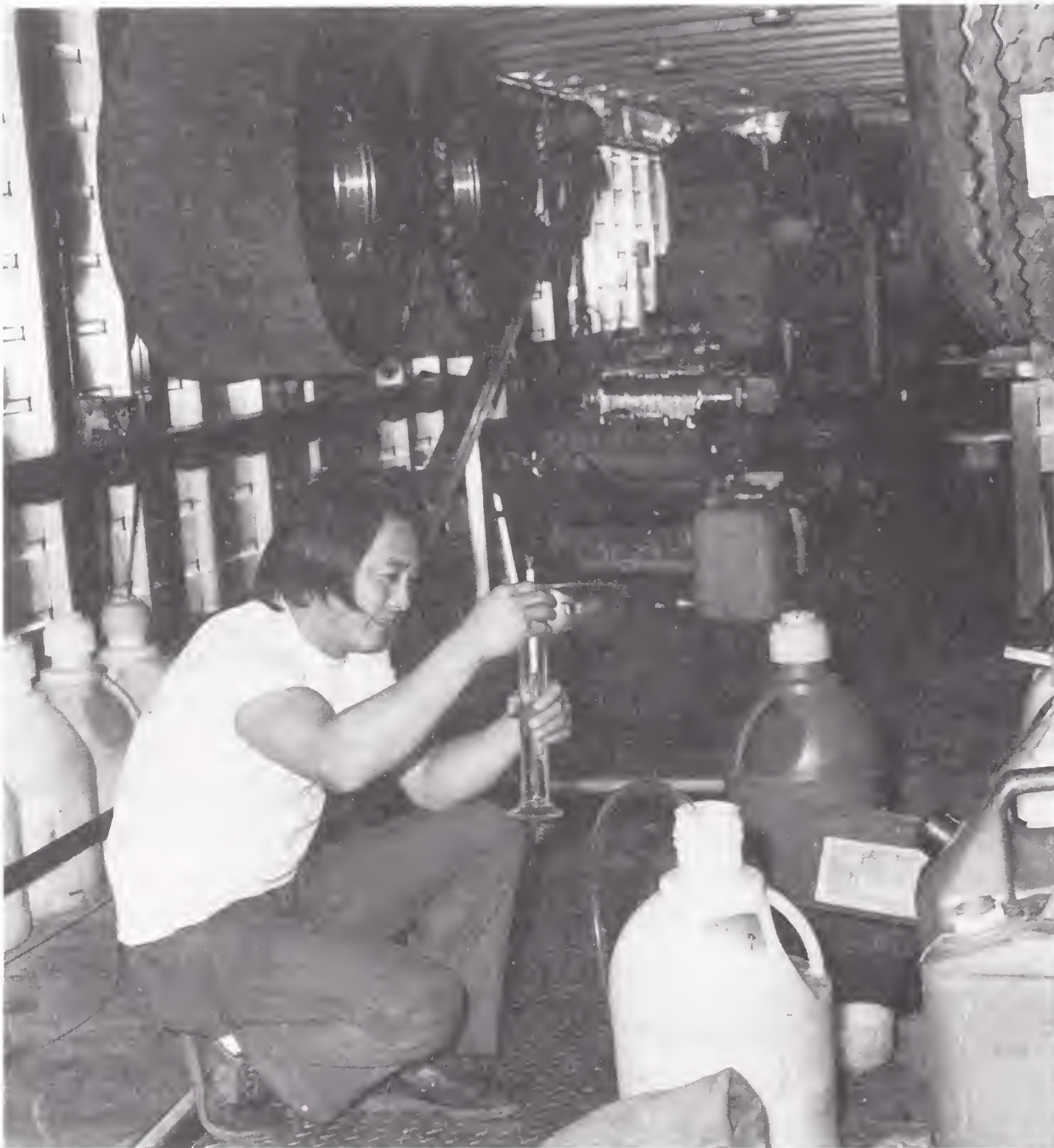
Dave Uyehara, seen here checking a fuel mixture with a hydrometer, drove dragsters and funny cars for many years while also operating a chassis fabrication shop. This photo shows the typical layout of a fifth-wheel trailer, with nitro in plastic containers arrayed low along the wall and spare wheels and tires hung up high. (Photograph by Leslie Lovett, courtesy National Hot Rod Assn.)
