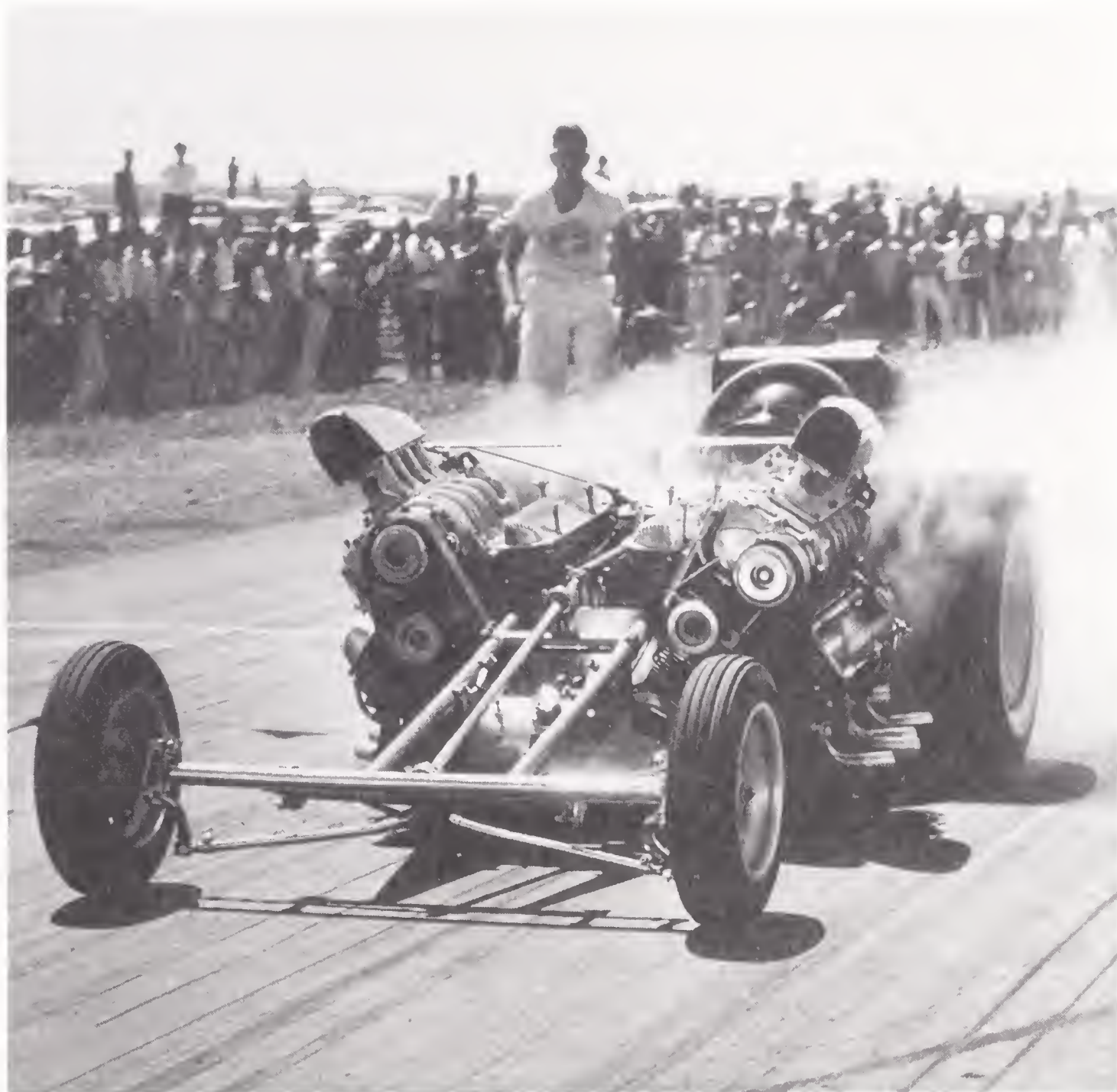
At an event at Amarillo Dragway prior to the 1961 NHRA Nationals, Eddie Hill charges off the line behind his twin Pontiacs. Hill was always an innovator; with this machine, in addition to everything else, the engines were integral with the frame. (Photograph by Don Brown, courtesy Museum of Drag Racing)
