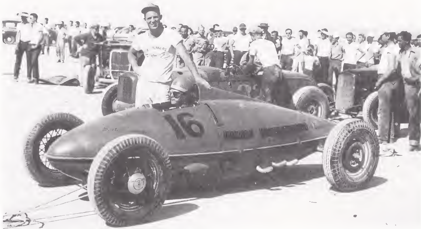
Bill Burke ran this machine at El Mirage from 1947 to 1949, and it was one of the featured attractions at the first Los Angeles Hot Rod Exposition. Lakesters configured like Burke's "Suite Sixteen," the bodies adapted from aircraft drop tanks, were thoroughly familiar to the first drag racers. (Photograph by Walt Woron, courtesy Museum of Drag Racing)
