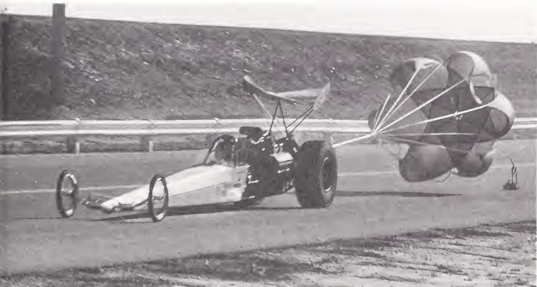
At Orange County an inadequately braced wing has given way, but this time the driver has the car under control and the chute safely out. (Photograph by John Shanks)
