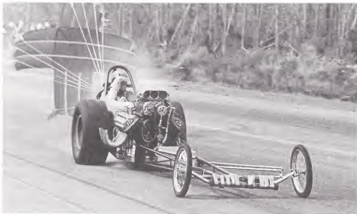
Bob Bofysil's slingshot was not unusual in the amount of weight it carried on the axle, although most racers were a little neater about how they attached it. (Photograph by Tim Marshall)
