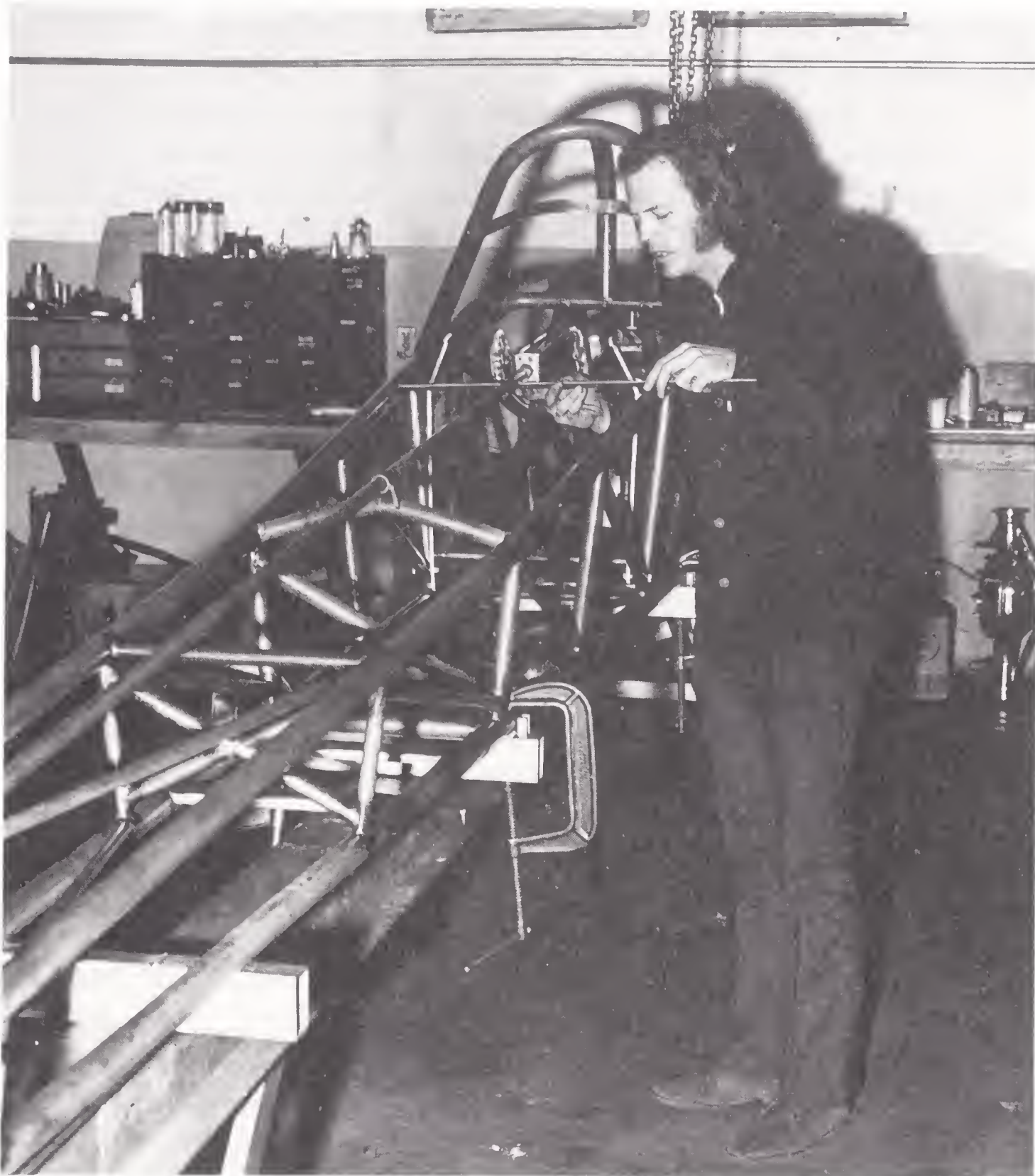
Fabricator Ron Attebury is seen here measuring to install the steering on a new chassis for Muldowney. Welding up a chassis on a jig like this assured that all components would be in proper alignment. (Author's collection)
