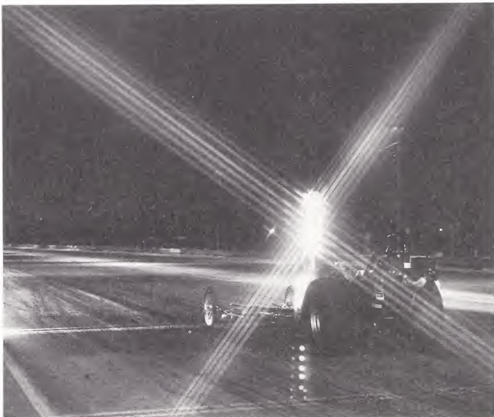
The instant before the big show: Lions Drag Strip, Long Beach, California, 1970. The photoelectric beam shining on Jim Dunn's spokes from the left indicates that he is staged. Not without reason are the starting lights called a Christmas tree. (Photograph by Mert Miller, courtesy National Hot Rod Assn.)
