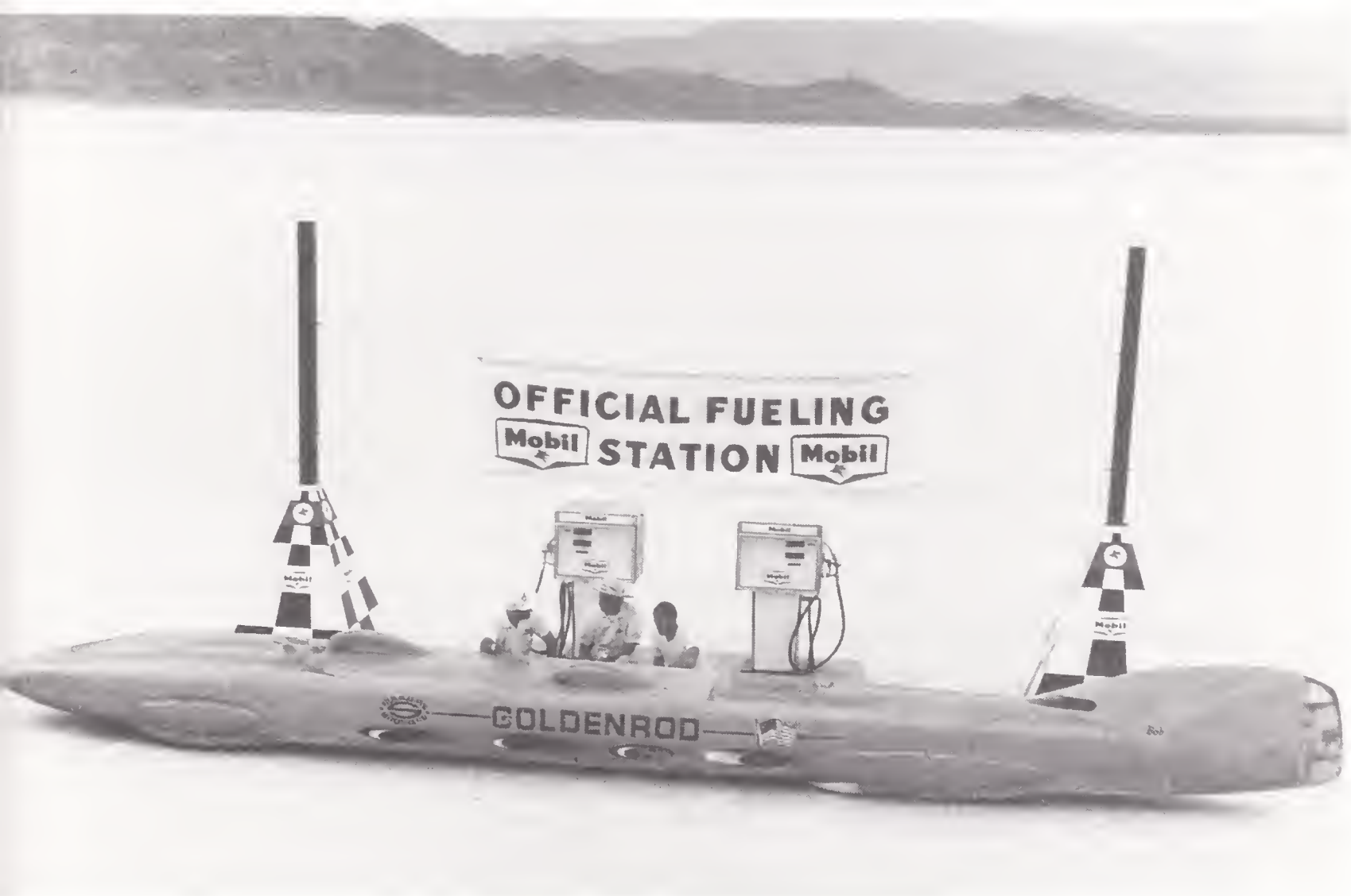
The Summers brothers' four-engine "Goldenrod," posed at Bonneville for a publicity photo in 1965. This machine was configured like a slingshot dragster but with a far superior Cd. It would hold the land speed record for piston engine power, 409.277, into the 1990s. (Photograph by Fred Wohlfarth)
