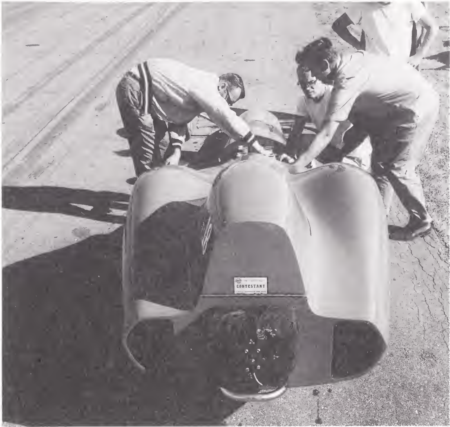
The Logghe-Steffey-Rupp streamliner from Michigan, like Breedlove's on the West Coast, had a K-form design aft, and it also had ample provisions for venting tire smoke. It is seen here being prepped for a run at the 1964 NHRA Nationals. (Photograph by Bob D'Olivo, courtesy Petersen Publishing Co.)
