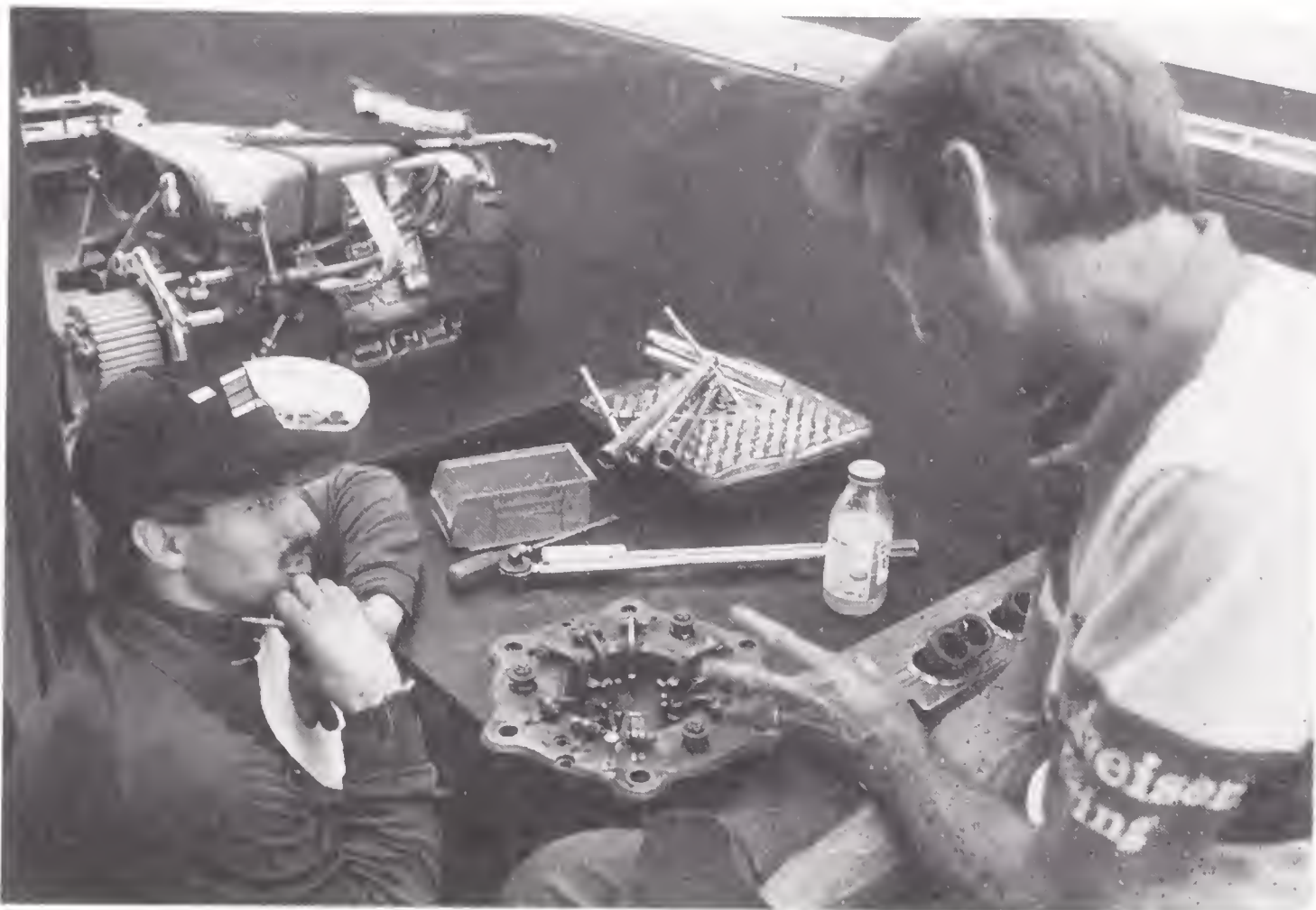
Dale Armstrong (right) confers with Lanny Miglizzi of L&T Clutches. The key to the L&T's "lock-up" feature was additional fingers on the pressure plate, the piece of hardware between them. On the next table is a blower and fuel injector. (Author's collection)
