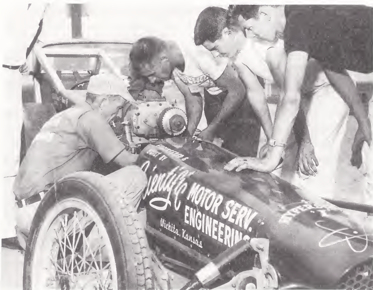
An inspector checks Al Williams’s “Hypersonic I,” a slingshot with a frame fabricated from rectangular aluminum tubing throughout (note the roll cage). Williams’s next machine was conventional chrome moly. (Photograph by Union Electric, courtesy Museum of Drag Racing)
