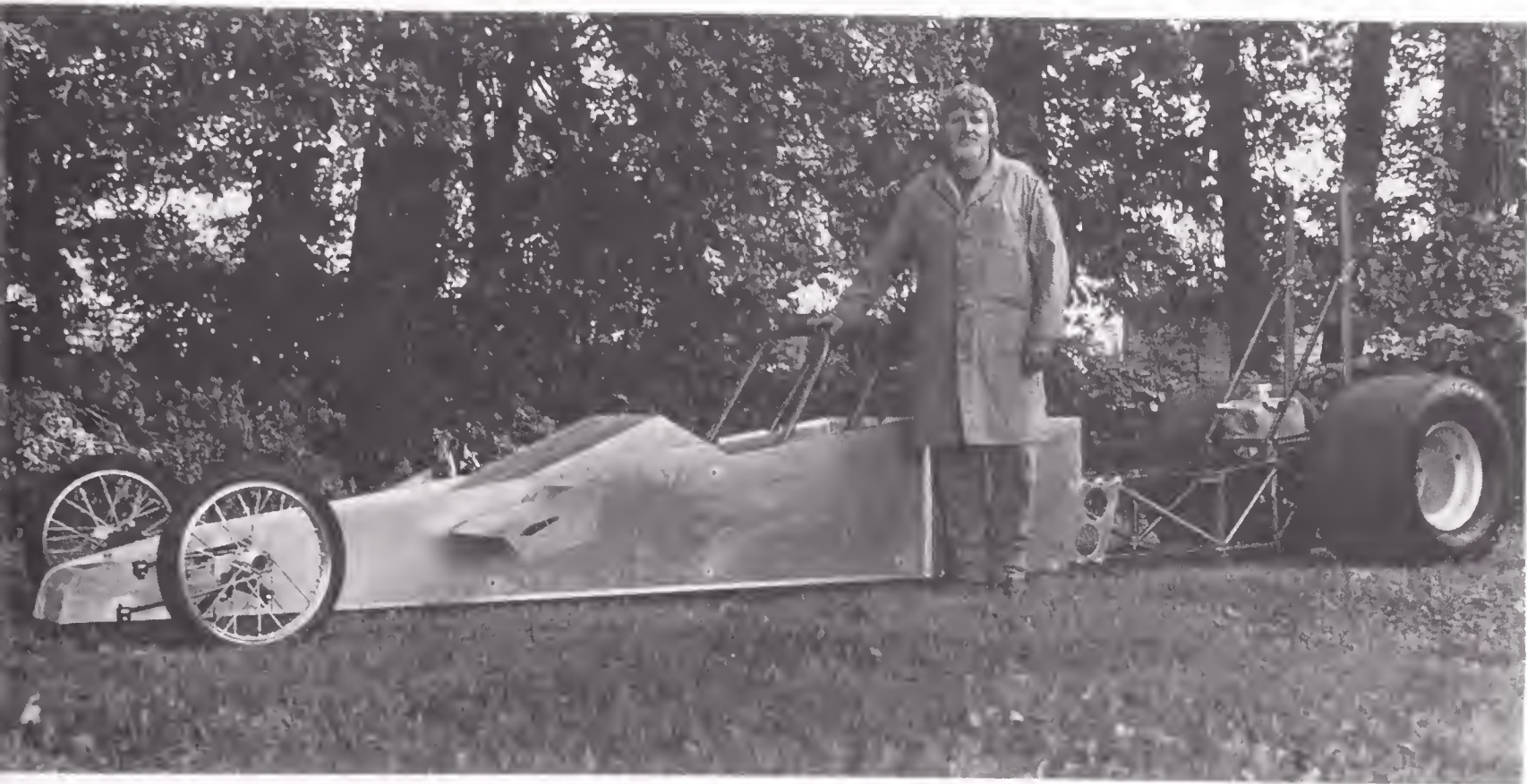
Dennis Rollain poses with the machine he built for Dave Miller in 1984; the wheel-base was 200 inches, when virtually every other top-fueler was five feet longer. (Author's collection)
