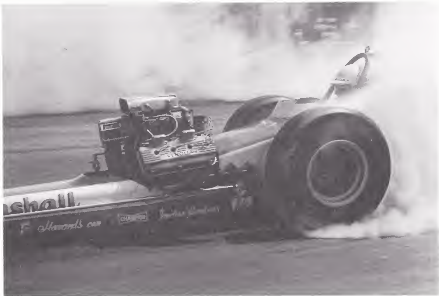
An inside joke. After having flipped over backwards, Rhode Islander Jim King rebuilt his slingshot and equipped it with a caster atop the roll bar, a precaution in the event of a recurrence. (Photograph by Ed Sarkisian)
