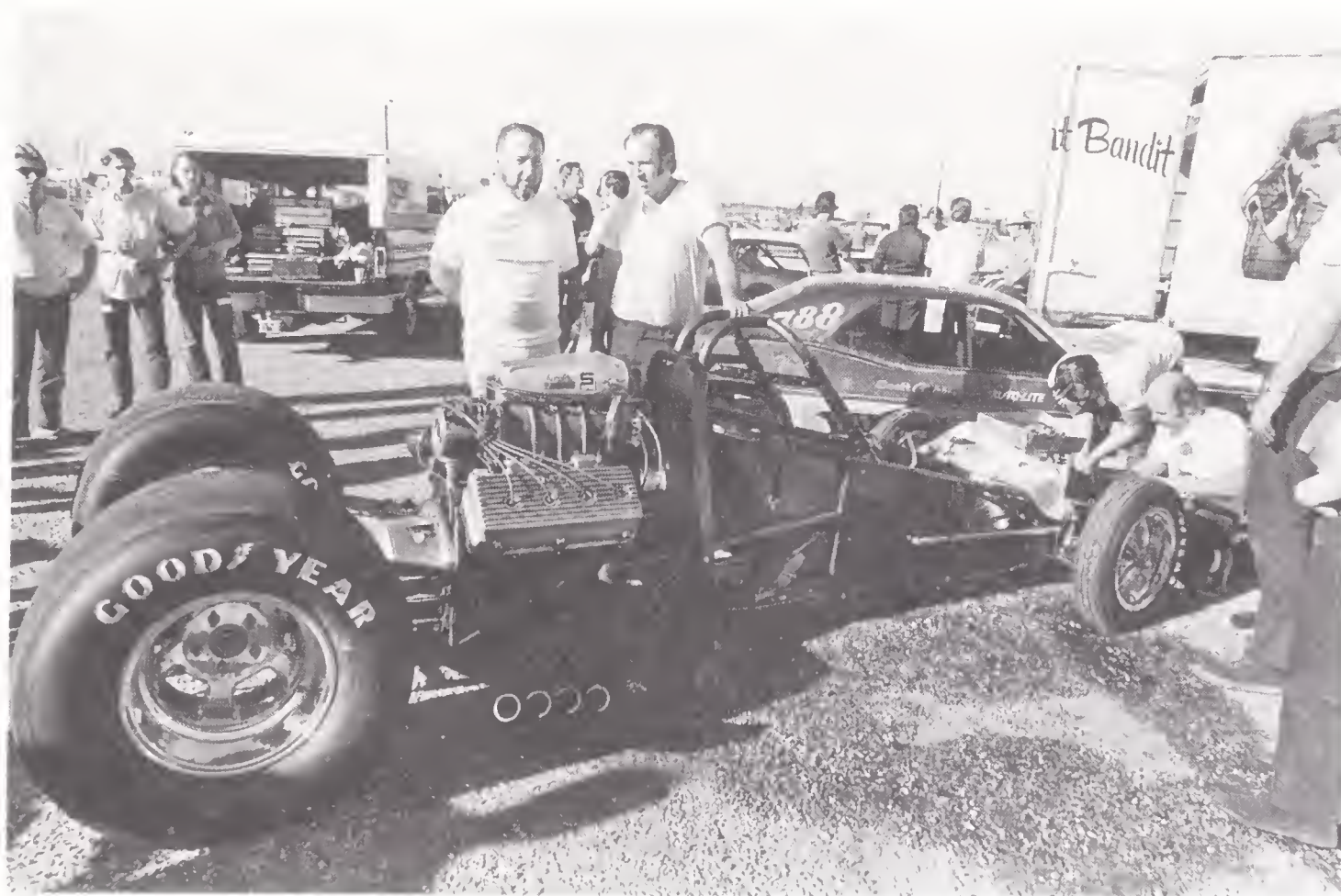
Woody Gilmore (left) poses with Jim Dunn and the mid-engine funny car he built for Dunn. The body is on the ground beyond them; Dunn drove with his face almost up against the windshield. (Author's collection)
