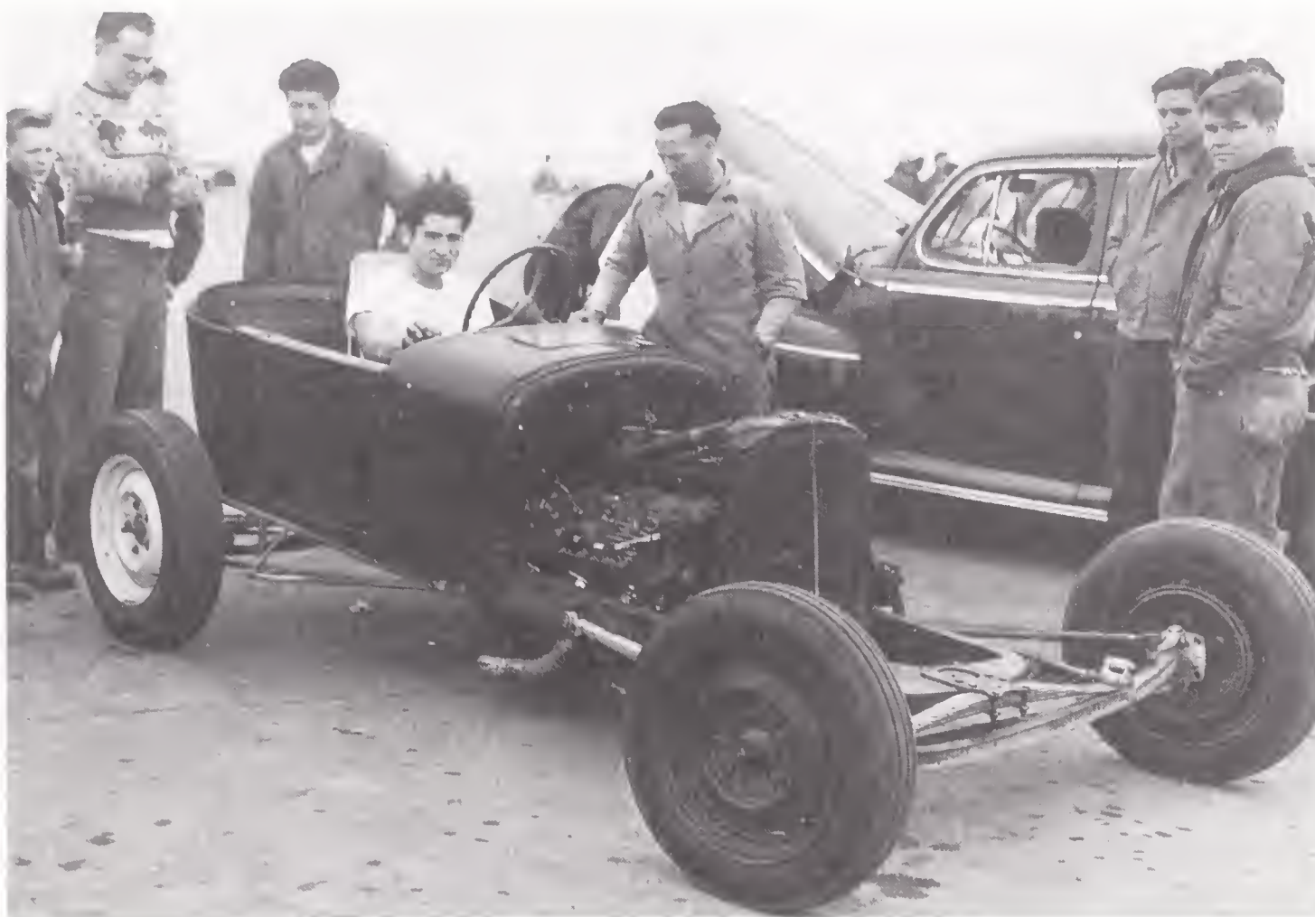
At Santa Ana, California, in 1950, Howard Johansen stands beside his stripped-down Model-T roadster. The engine is a Ford V-8 with three carburetors and finned aluminum heads. In coveralls behind driver Ed Osepian is Nick Arias, Jr., who, like Johansen, would become a prominent manufacturer of this kind of equipment. (Courtesy National Hot Rod Assn.)
