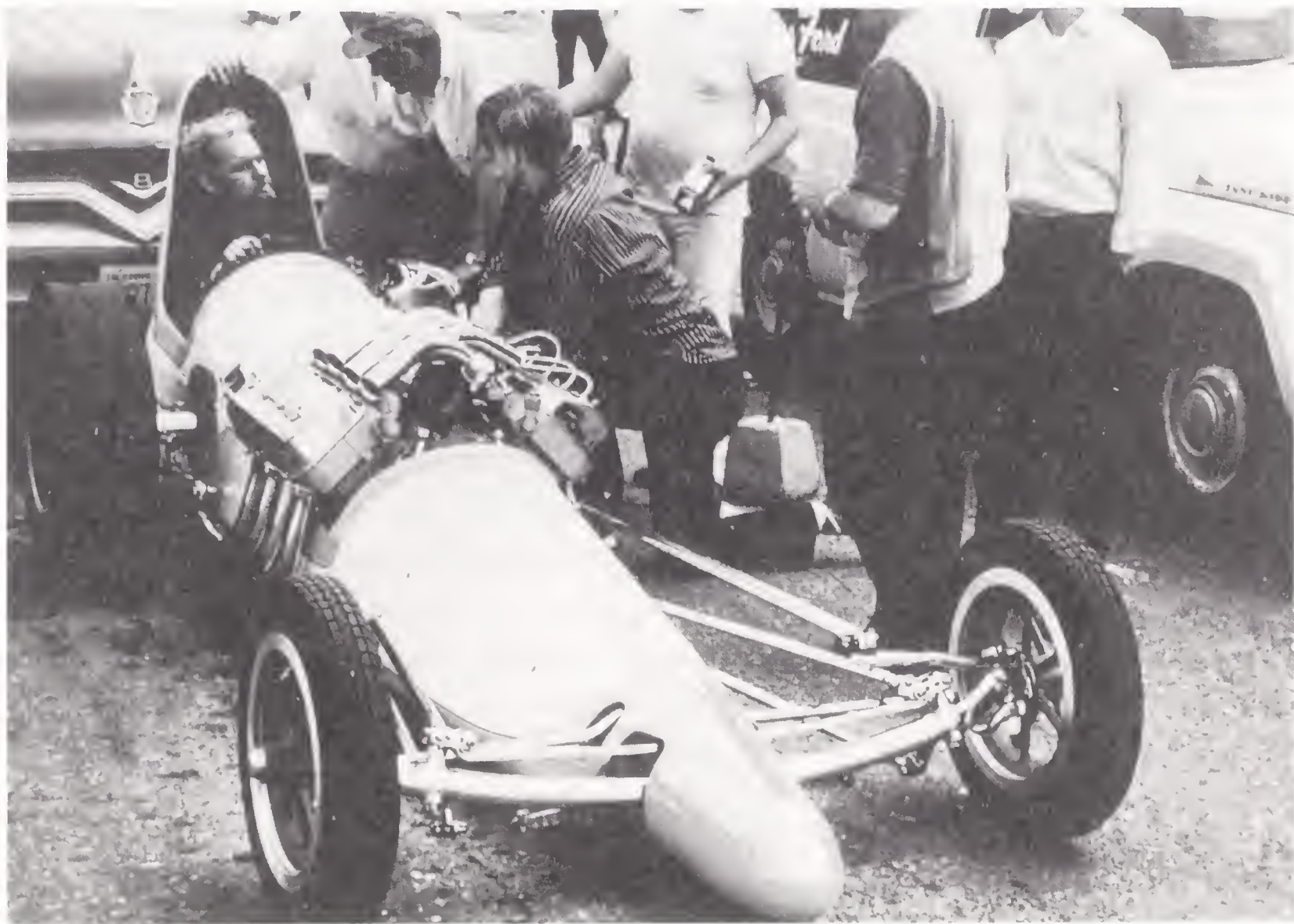
Besides the obvious differences, such as fuel injectors rather than carburetors, contrast the detailing of Romeo Palamides's machine with Garlits's (facing page). Here Pete Ogden is seen in the cockpit. (Courtesy Don Jensen)
