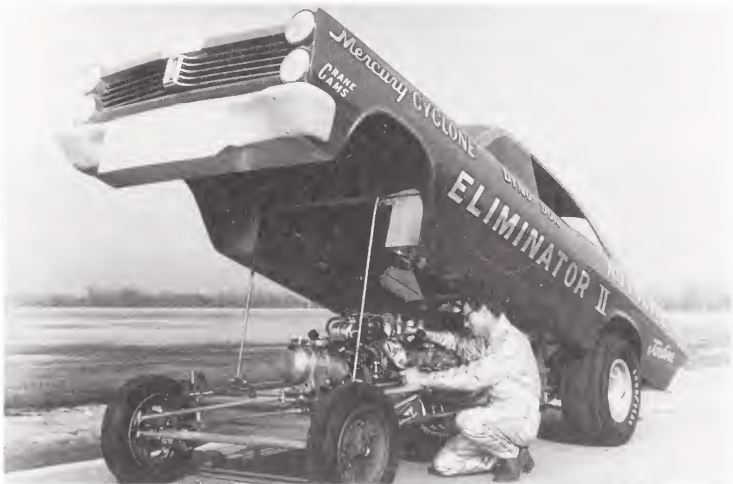
Don Nicholson poses with one of the machines built in 1966 by the Logghe chassis shop in Michigan. This "flip top" means of access to the engine and cockpit inspired the sobriquet "flopper." (Courtesy Lincoln-Mercury Division, Ford Motor Co.)
