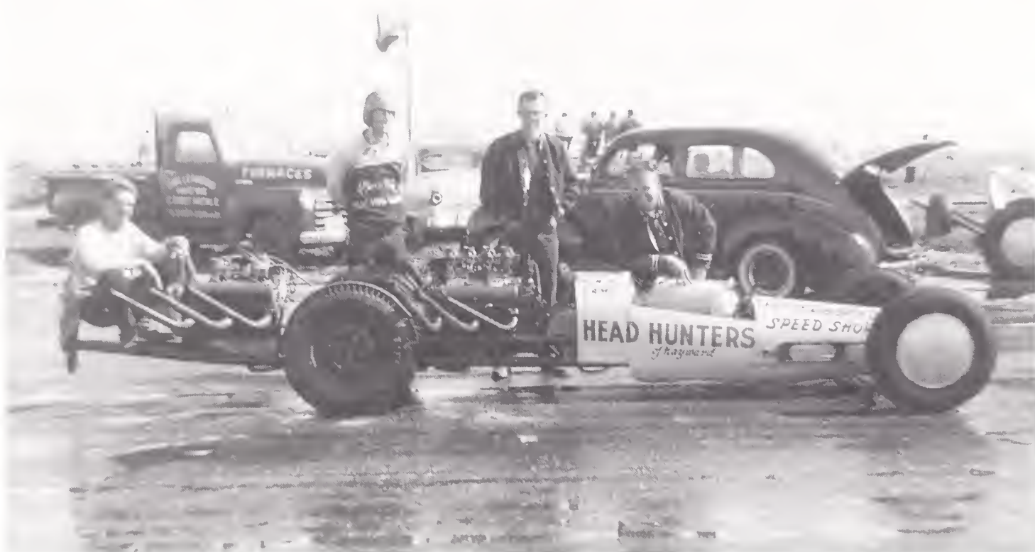
Don Jensen's twin-engine machine of 1956, which combined the cockpit location of a modified roadster with a rear engine like the Bustle Bomb. In this shot Jensen is seated on the edge of cockpit. On his right are members of his Hayward, California, club, George Wulf (who owned the rear engine), Donn Blount, and Bryan Burnue. (Courtesy Don Jensen)
