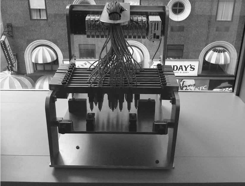
FIGURE 1.2. Lehman Brothers “Clackatron” (ca. 2002), used to strike the keys of an EBS (Electronic Broking Services) foreign-exchange trading keypad. Photograph courtesy of interviewee FL.
