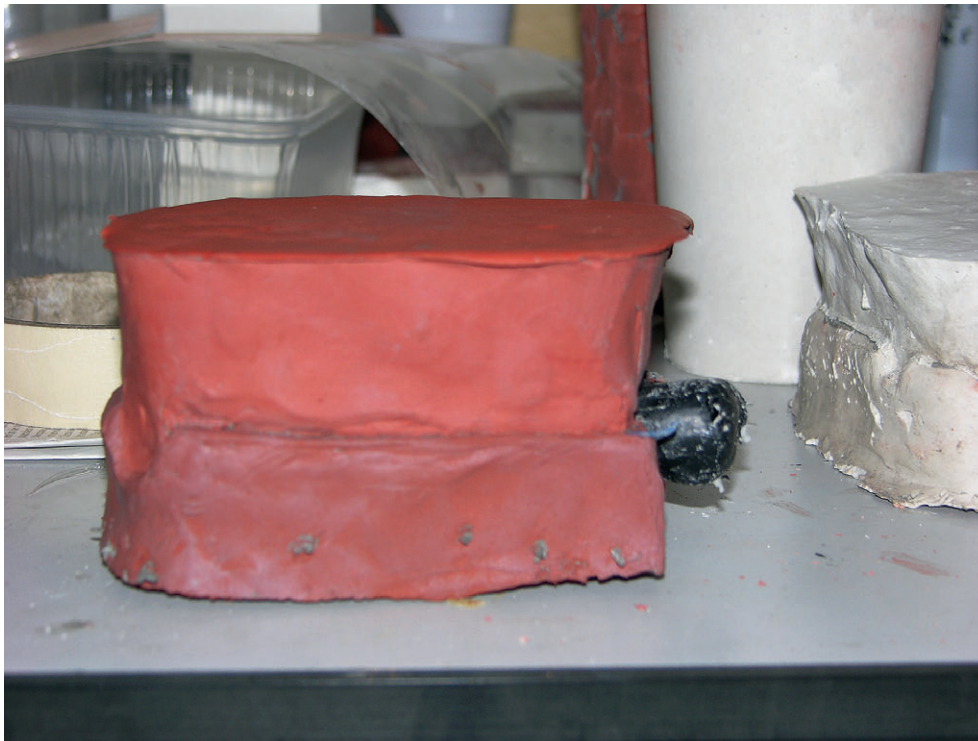
10.1. A deep red, two piece mold following recipes in Ms. Fr. 640 for combining plaster of Paris, ground and previously fired molds, ground bricks, water, iron oxide, ammonium chloride, and eggs. Created by Pamela H. Smith and Tonny Beentjes. Photo: Pamela H. Smith and Tonny Beentjes.
