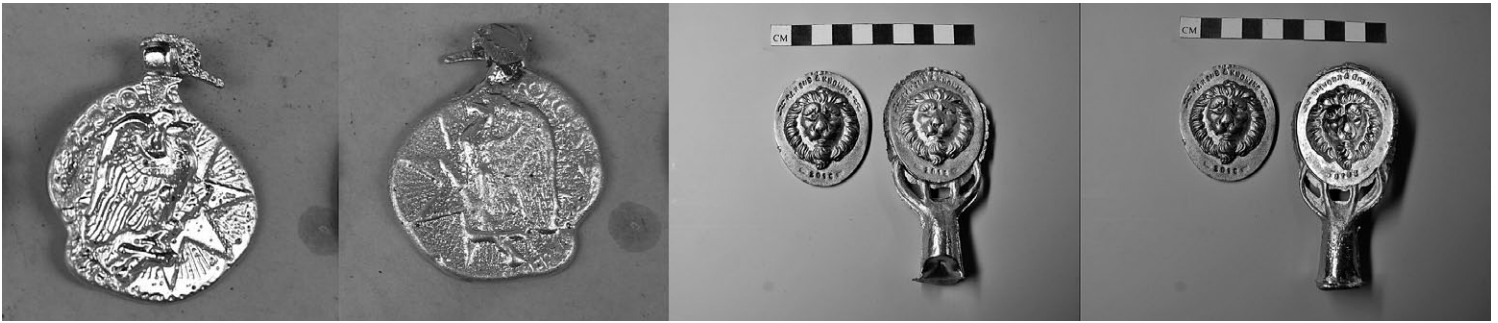
9.11. Collaboration between the Making and Knowing Project and the University of Amsterdam Metalwork Conservation Program on Ms. Fr. 640, fol. 92r, “Molding hollow on one side and in relief on the other.” Left to right: Making and Knowing team members Rozemarijn Landsman and Jonah Rowen, “proof of concept,” cast tin medal: concave side, convex side. University of Amsterdam team members Michaela Groeneveld and Marianne Nuij, cast tin medal: pattern, convex side; pattern, concave side. © Making and Knowing Project. CC BY NC SA.
