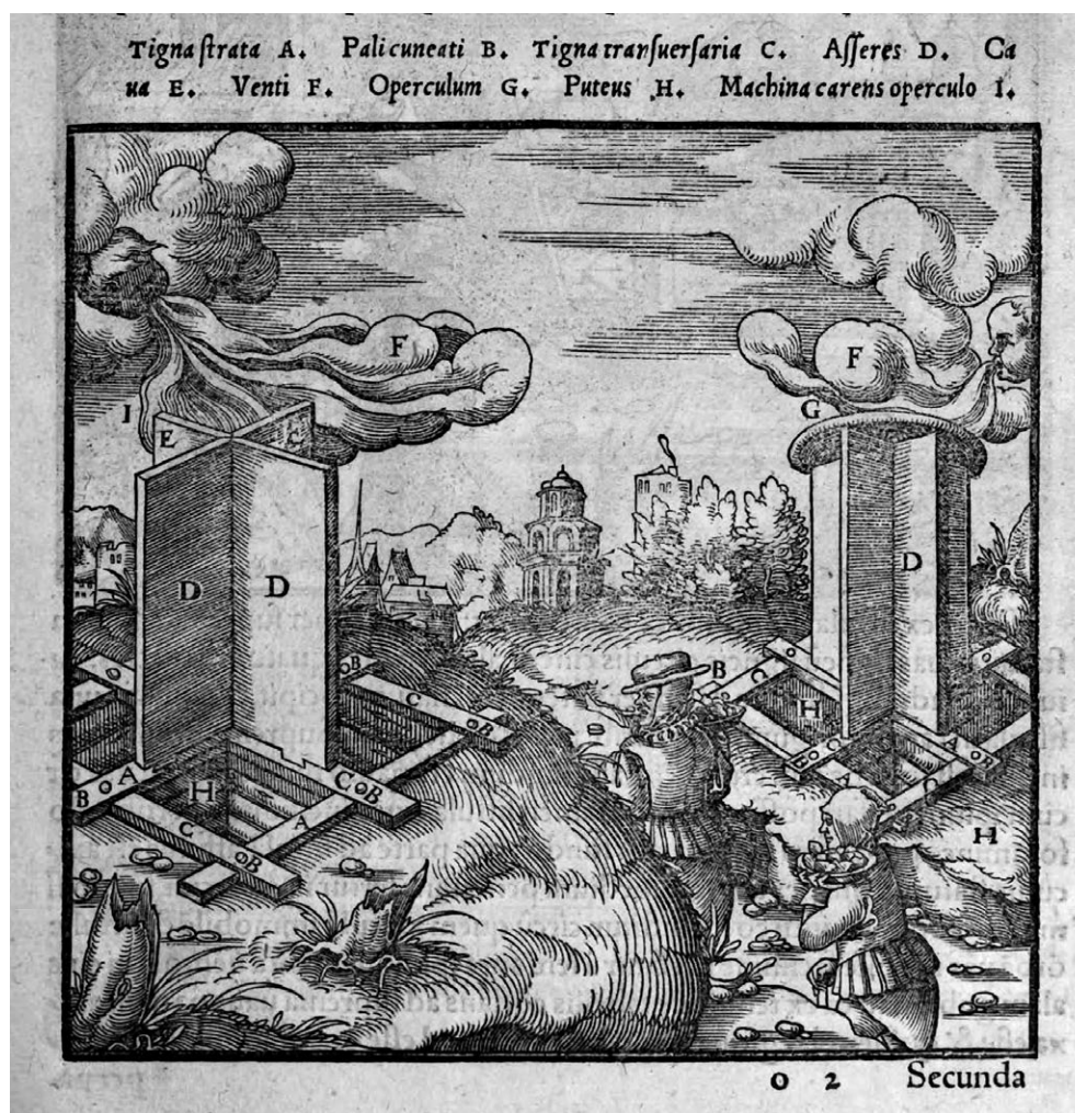
4.13. Georgius Agricola, De re metallica: libri XII (Basil: Froben, 1561), book 6, p. 159. Aboveground fans intended to bring air into the mine shafts. Bayerische Staatsbibliothek, Munich, Res/BHS II B 5#Beibd.1. Notice the analogy between the older classical structures in the distance and the new mine ventilation towers in the foreground. http://mdz.nbn-resolving.de/urn:nbn:de:bvb:12-bsb10199044_2 .
