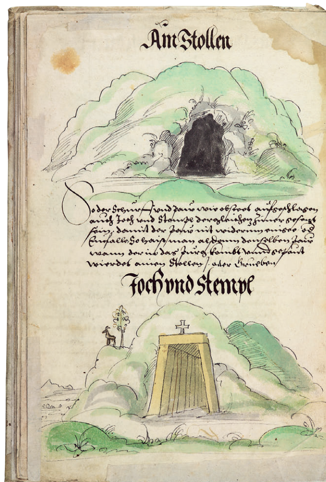
2.5. Ain Stollen (an adit, or shaft entrance) and Joch und Stempel (a reinforced shaft), from Schwazer Bergbuch , Bochumer Entwurfs exemplar (1554), p. 16. From the 1554 draft of the Schwazer Bergbuch , this illustration shows the shaft opening before and after being shored up. Reinforcing the mine shaft included making a cross over the entrance. Montan historisches Dokumentationszentrum beim Deutschen Bergbau Museum, Bochum, 040003313001. © Deutsches Bergbau Museum.
