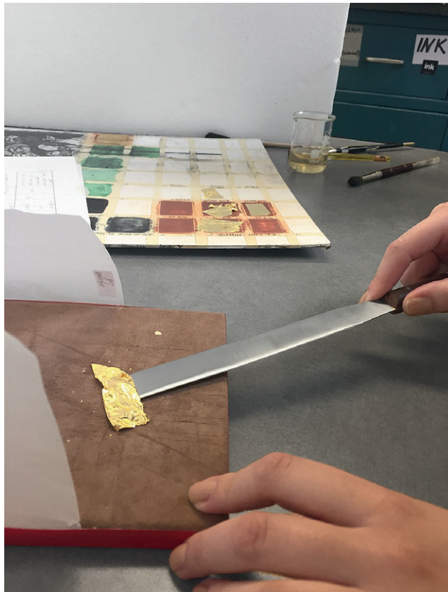
9.8. Marjolijn Bol led the laboratory seminar students in creating a panel with a historically authentic gesso ground. The panels then served the students in testing and practicing painting and gilding techniques. © Making and Knowing Project. CC BY NC SA.
