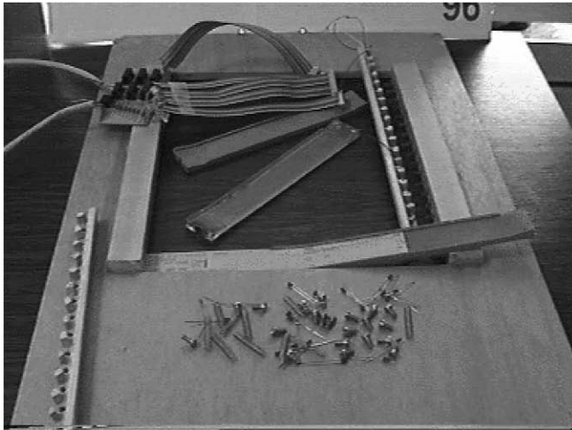
FIGURE 52.15. Caméléon's augmented stripboard (left) is a working hardware prototype that identifies and captures hand-writing from paper flight strips. Members of the design team test the system (right), which combines both hardware and software prototypes into a single interactive simulation.
