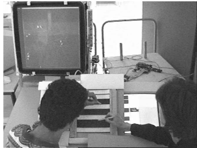
FIGURE 52.15. Caméléon's augmented stripboard (left) is a working hardware prototype that identifies and captures hand-writing from paper flight strips. Members of the design team test the system (right), which combines both hardware and software prototypes into a single interactive simulation.
