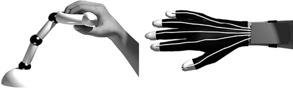
Figure 20.5 End-effector (left) and generic full-hand exoskeleton (right)
