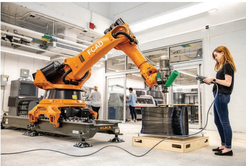
0.3 The Creative School Design + Technology Lab – Kuka robot with custom 3d printing tooling. Courtesy of The Creative School Design + Technology Lab
