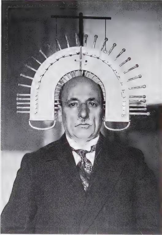
Cephalometer, used for precise skull measurements for body-type and phrenological classification purposes. Photograph courtesy Museum voor Communicatie, The Hague.
