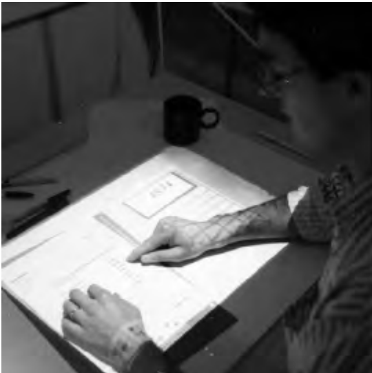
Figure 2.3 Wellner's Digital Desk allowed interaction with paper and electronic documents on the same desktop. Reprinted by permission of Xerox Research Centre Europe.
