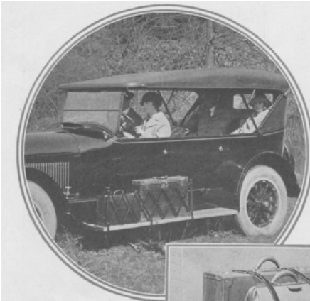
Having end guards and being attachable by malleable clamps and thumb screws, the carrier shown in the drawing below securely holds one or several pieces of luggage to the running board.
