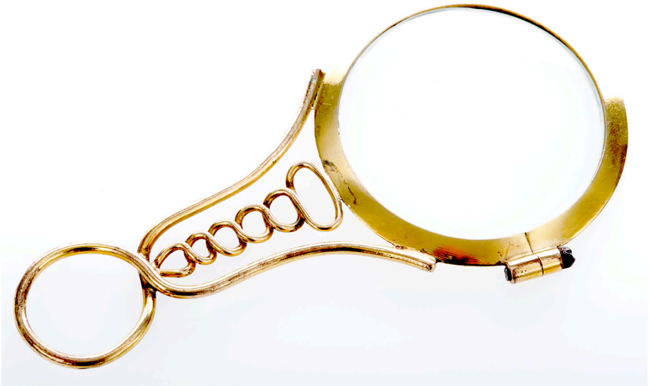
Figure 10 Quizzing glass to be held in the hand close to the eye in order to view distant objects, featuring a gold frame with a bevelled lens rim. The handle is comprised of two curving pieces and multiple oval loops and features a suspension ring at the end. French, c.1820. British Optical Association Museum, Catalogue number LDBOA1999.3776. © The College of Optometrists, London.
