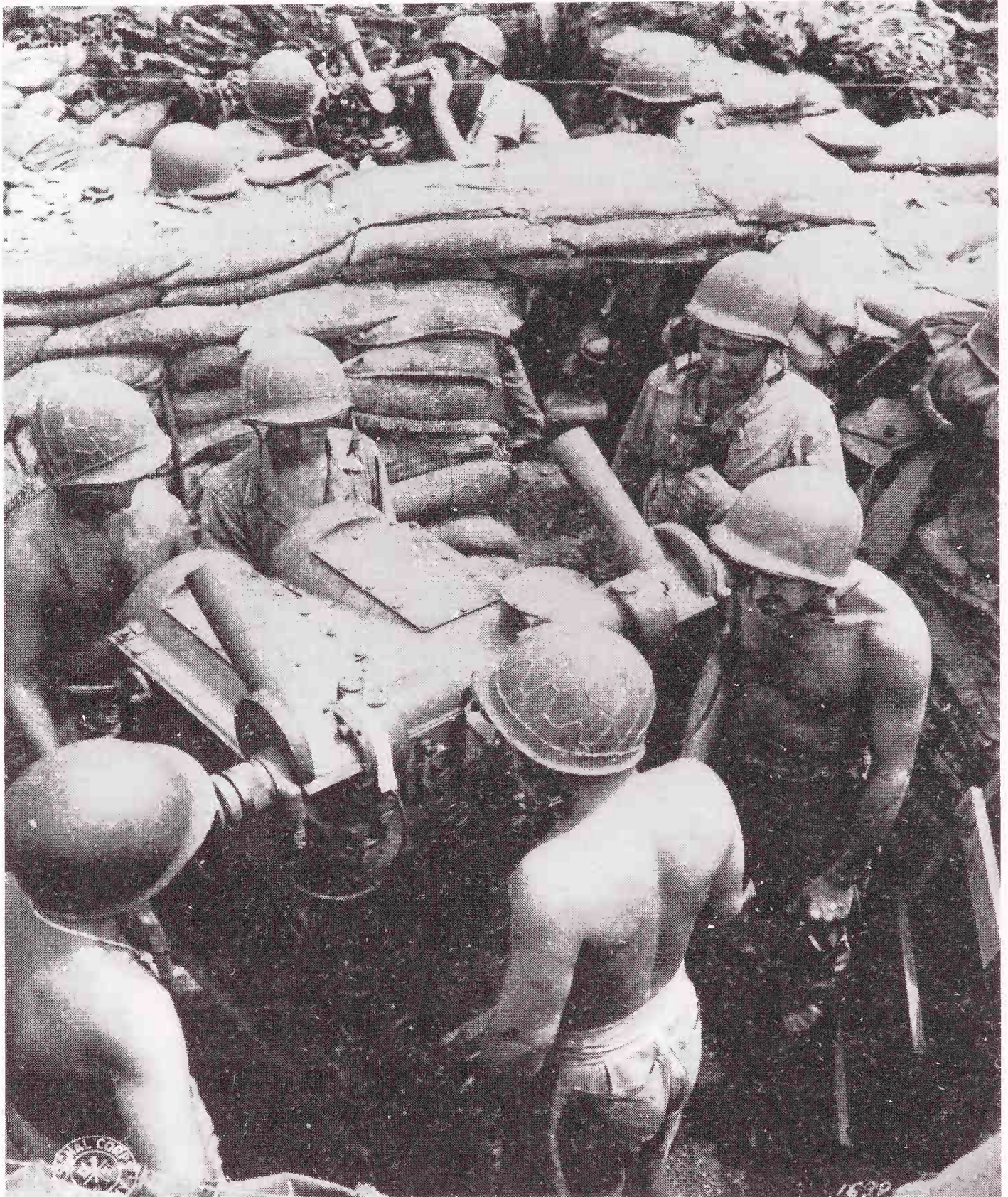
Soldiers using a Sperry M7 analog antiaircraft gun director during World War II. Courtesy Sperry Corporation Collection and the Hagley Museum and Library.
