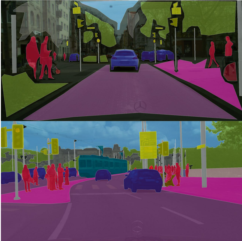
Fig. 3.1 Difference between coarse (top) and fine (bottom) annotations in the Cityscapes Datasets. (Source: Cityscapes, 2022)
