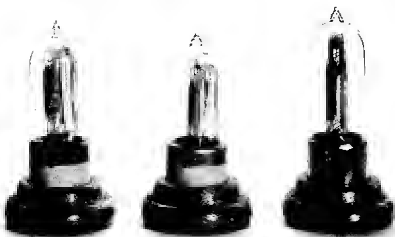
Fig. 6-19. Successive steps in the transformation of the early Type J tube into a rugged unit, suitable for military applications.
