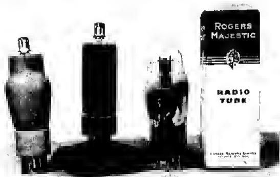
Fig. 17-23. Rogers Types 88S, 88M, and Rogers-Majestic Type 27 with carton. Left to right: 88S with spray shield, 88M with black "metallized" coating, and Rogers Majestic Type 27 with carton.
