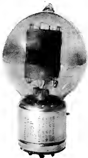
Fig. 6-23. The 205B vacuum tube. The same as the VT-2 except for markings.
