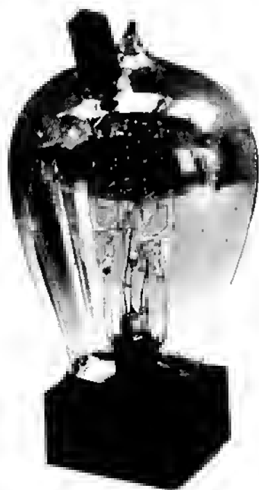
Fig. 8-4. An early type of wire-element Plotron, now in the Science Museum, London.
