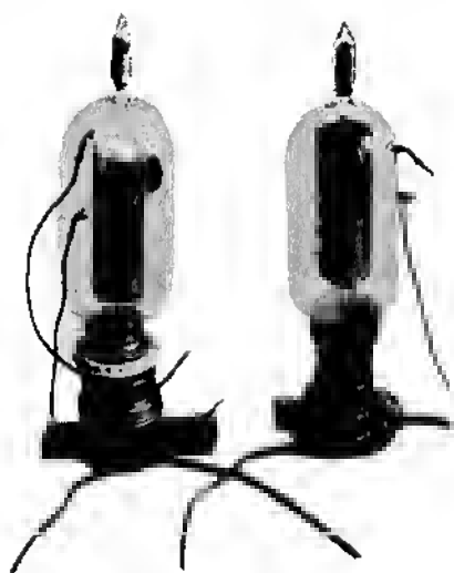
Fig. 11-8. Left: Round Type N with Edison medium screw base. Right: Round Type N with Edison bayonet base.
