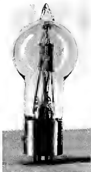
Fig. 9-17. The de Forest singer-type tube, 1920.
