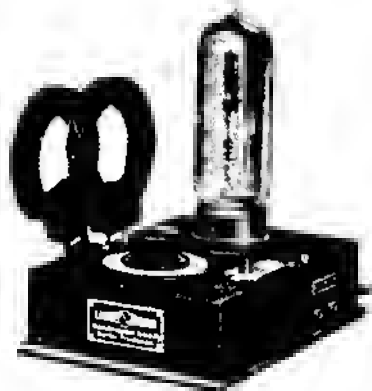
Fig. 21-27. Loewe Type OE333 radio receiver using 3NF tube. (Reproduced from Wireless Mag. , Dec. 1927.)
