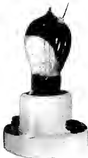
Fig. 4-3. Fleming valve made for C. D. Babcock by McCandless & Company in latter part of 1905.
