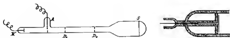
Fig. 2-11. Drawing of Zenneck's modification of the Braun tube. The tube assembly is at left, and details of the cathode at right. (Reproduced from Ann. Phys. , 1899, 69.)
