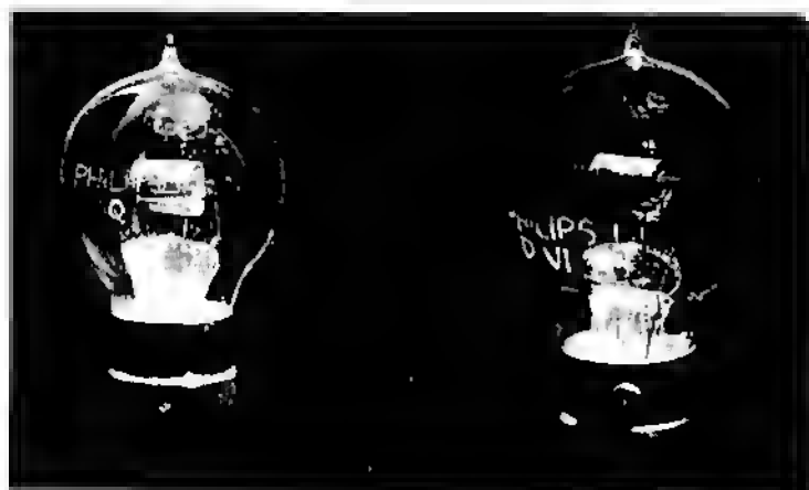
Fig. 20-6. Philips Q and D VI tubes. Tubes are the same but bear different markings. The Q is the earlier marking.
