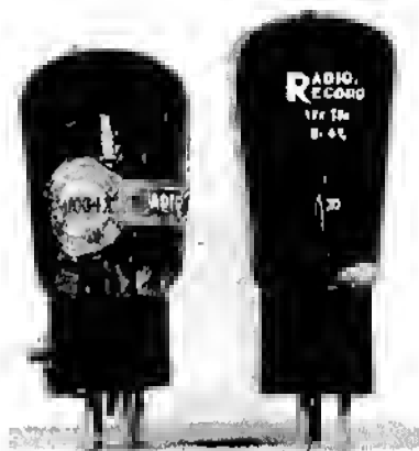
Fig. 20-18. Radio Record tubes. Left: M1004X. Right: RRR134.
