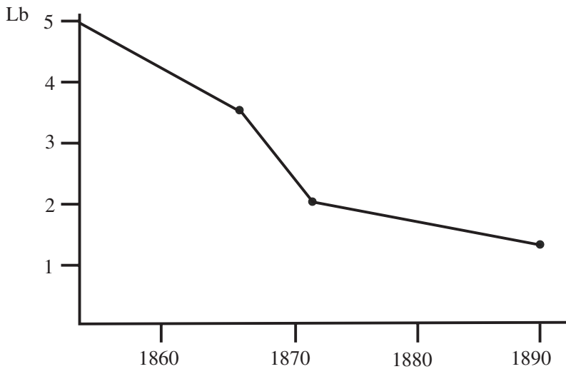
Figure 4.10 Coal consumption of marine steam engines (lb per indicated hp/hr)
